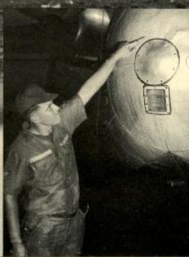
Airman points to patched bullet holes in Ranch Hand UC-123. Aircraft has taken 546 hits since arriving in Vietnam in 1962.
